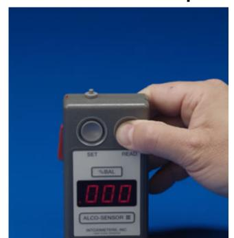
**Step 6: Zero Check** If .000 is not seen in the bright mode, press SET button and recheck in one minute.
