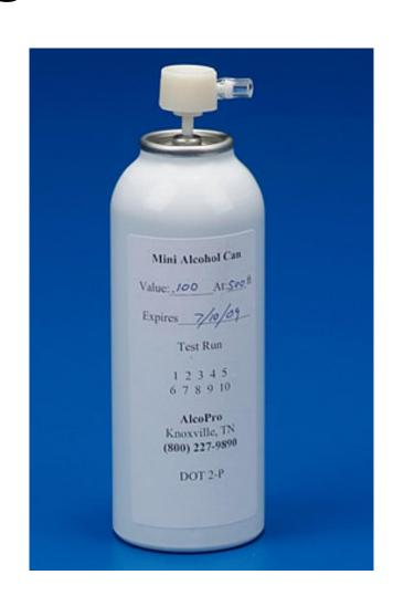
**Step 1: Mount Regulator** Remove the protective vinyl tubing from the top of the Mini Can, as shown in the 1st picture, and discard the tubing. Then install the valve as shown in the second picture.
