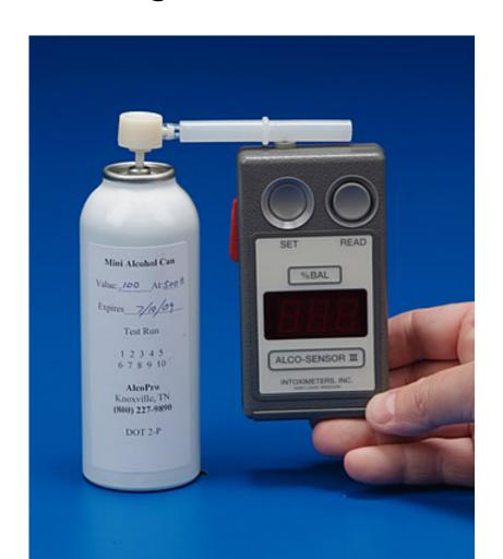
**Step 9: Sample Gas** Press the Mini Can valve for 4 seconds. On the 3rd second of the 4-second count, depress the READ button. (NOTE: The gas must be flowing through the mouthpiece when the READ button is depressed).
