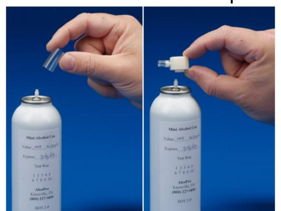
Step 2: Target Value Note the "Value" printed on the can. In this case, the Value is .100. This will be the target value.
